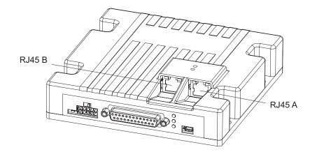
FIGURE 8. Ethernet Ports location
