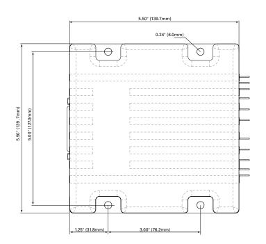
FIGURE 14. FBLG2360T top view and dimensionsMechanical Specifications
