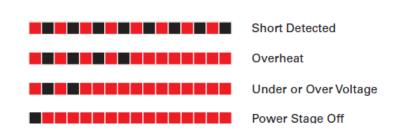
FIGURE 10. Exception or Fault Flashing Patterns
