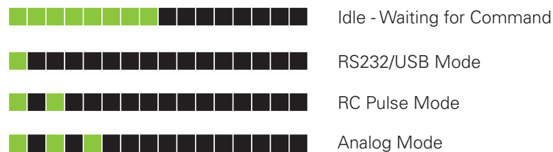
FIGURE 11. Normal Operation Flashing Patterns
