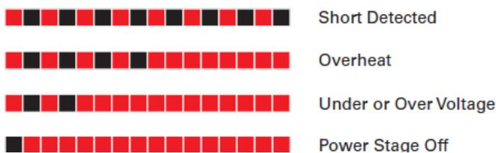
FIGURE 10. Exception or Fault Flashing Patterns
