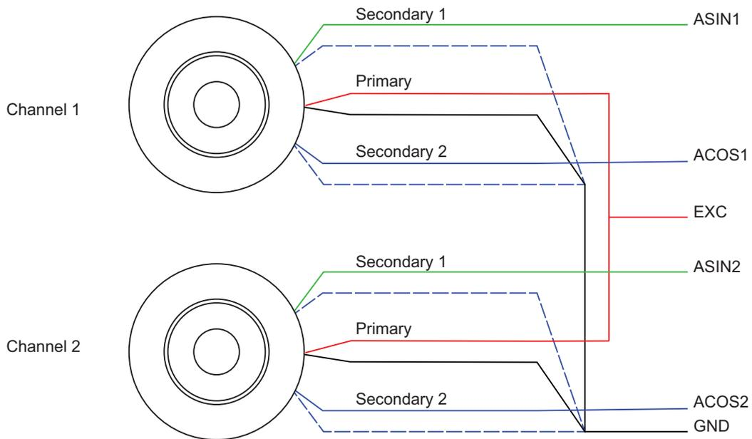
FIGURE 6. Resolver wiring
