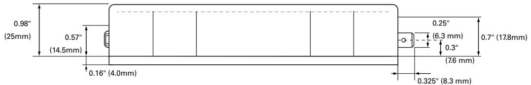
FIGURE 13. FBLG2360T side view and dimensions
