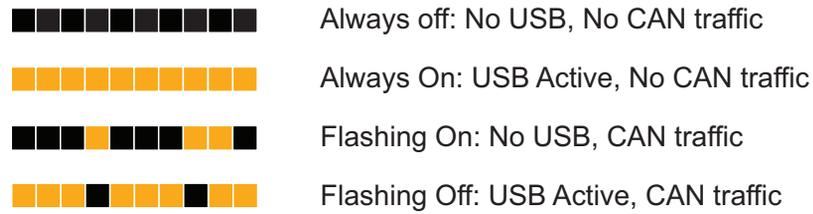
FIGURE 11. Exception or Fault Flashing Patterns
