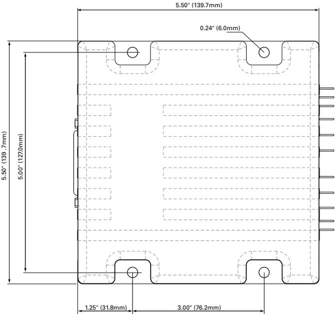
FIGURE 14. FBLG2360T top view and dimensions Mechanical Specifications
