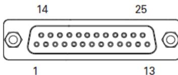
FIGURE 7. Main Connector pin locations
