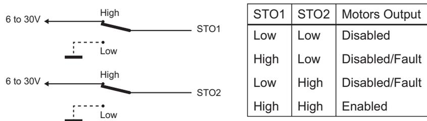
FIGURE 12. STO input levels effects on controller output
