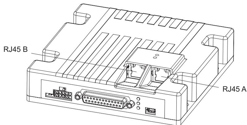
FIGURE 8. Ethernet Ports location
